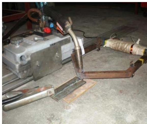
Fig 4. Setting up electromagnet and welding torch with the auto feeding device.
